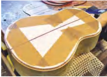
STEP 39. Using parcel tape, as shown, helps to ensure a tight grip
